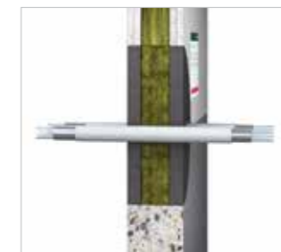
Wall penetrations with composite plastic pipes including aluminium up to Ø32 mm EI 120 U/C.
