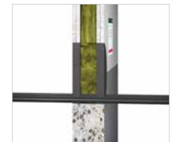
Wall penetrations with sheathed cables up to 21 mm or cable bundles up to 50 mm EI 120.
