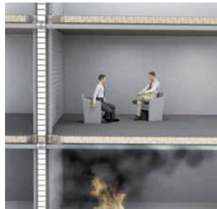
1. Fire breaks out in a fire compartment
