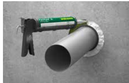
4. Seal the gap with Pacifyre® A Acrylic Sealant (t = 10 mm).
