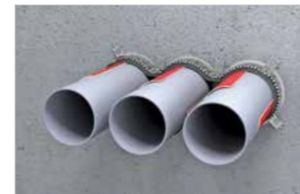
■ Multiple penetrations (max. 3 pipes through 1 Fire Collar). Distance between pipes ≤ 15 mm.
