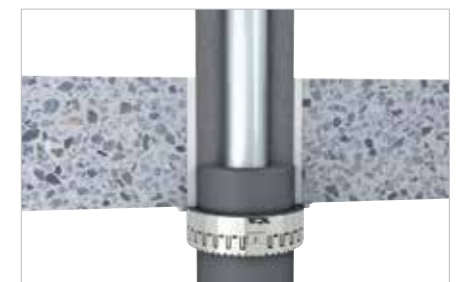
■ Non-combustible pipes with a collar on the underside of the floor.
