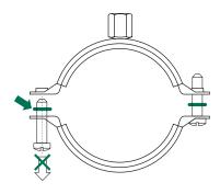
Anti-loss washers prevent screws from falling out
